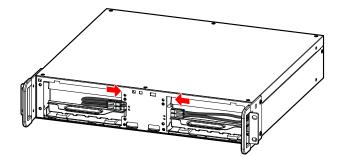
Step 7 Install the battery plate.
