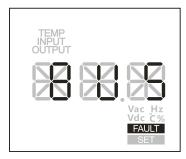
Figure2-23 Busbar voltage fault
