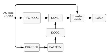
Figure 2-8 Work principle of 1-3kVA(L)
