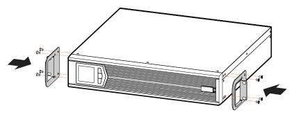
Figure3-1 Install angle iron
