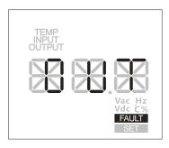
Figure2-26 Output fault
