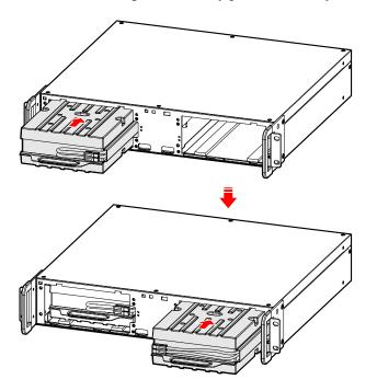
Step 6 Plug the battery wire.
