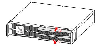
Step 9 Finish battery pack installation.
