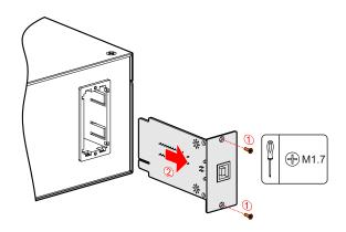
Step 2 Install optional intelligent slot and fix it.
