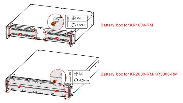
Step 8 Install the left and right plastic panel.
