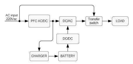
Figure 2-9 Work principle of 6kVA(L), 10kVA(/B)
