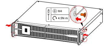
Step 3 Fix battery box (optional) on the rack.
