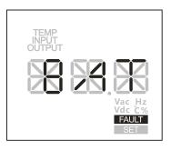
Figure2-27 Battery fault
