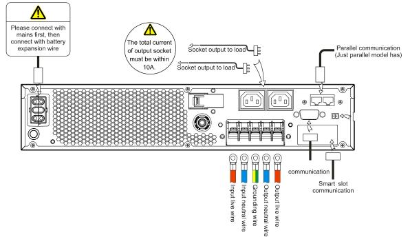
Figure3-5 Wiring diagram of 6kVA(L), 10kVA (/B)
