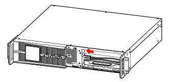
Step 7 Install the battery plate.
