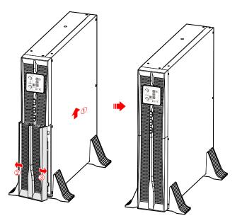
Step 4 Place UPS with support bases, and then install the plastic panel.
