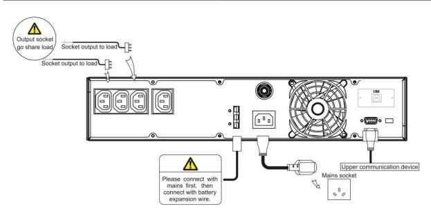
Figure 3-3 Wiring diagram of 1kVA(L)
