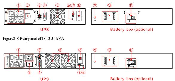
Figure 2-9 Rear panel of IST3-J 2kVA / IST3-J 3kVA
