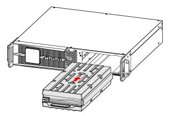
Step 6 Plug the battery wire.
