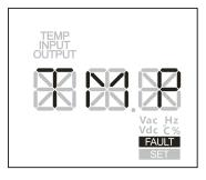
Figure2-24 IGBT over-temperature fault
