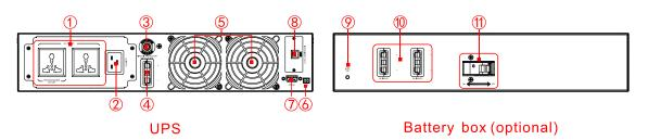
Figure2-15 Rear panel of IST3-J 2kVA/ IST3-J 3kVA
