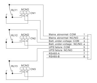
Figure 2-7 Pin definition of RS485 and dry contact
