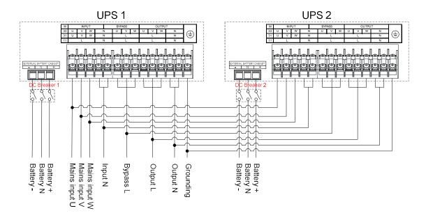
31 mode parallel system wiring diagram of IST7 10-20KVA
