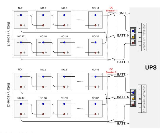
Wiring diagram 3 of external batteries
