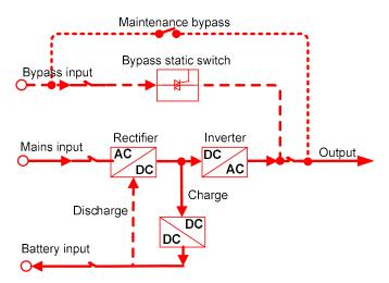
Normal mains power supply mode (the thick solid line stands for the energy flow direction)
