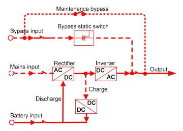
Battery inverter mode (the thick solid line stands for the energy flow direction)
