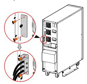
Extension battery wiring assembly of IST710
