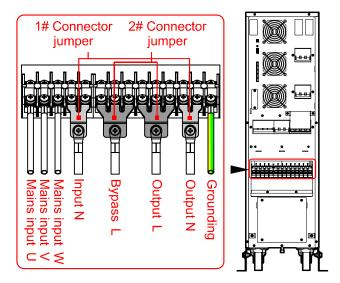
Connector jumper and wiring diagram of 31 mode
