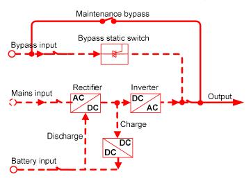
Maintenance bypass power supply mode (the thick solid line stands for the energy flow direction)
