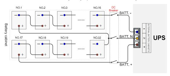
Wiring diagram 1 of external batteries
