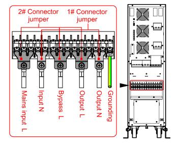
Connector jumper and wiring diagram of 11 mode
